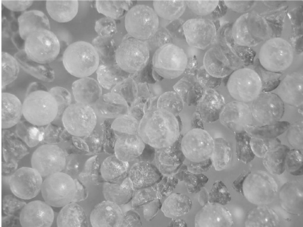
FIGURE 7.31 Sample resin #1 exhibits a moderate fouling with organics with a high percentage of broken beads.
