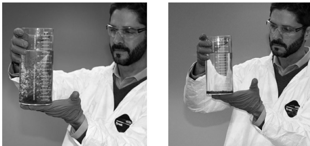
FIGURE 6.14 Cylinder test showing the stages of mixing and settling.
